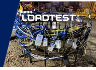
Fugro LOADTEST has been performing Thermal Integrity Profiling on both preliminary and working foundation elements for many years.
